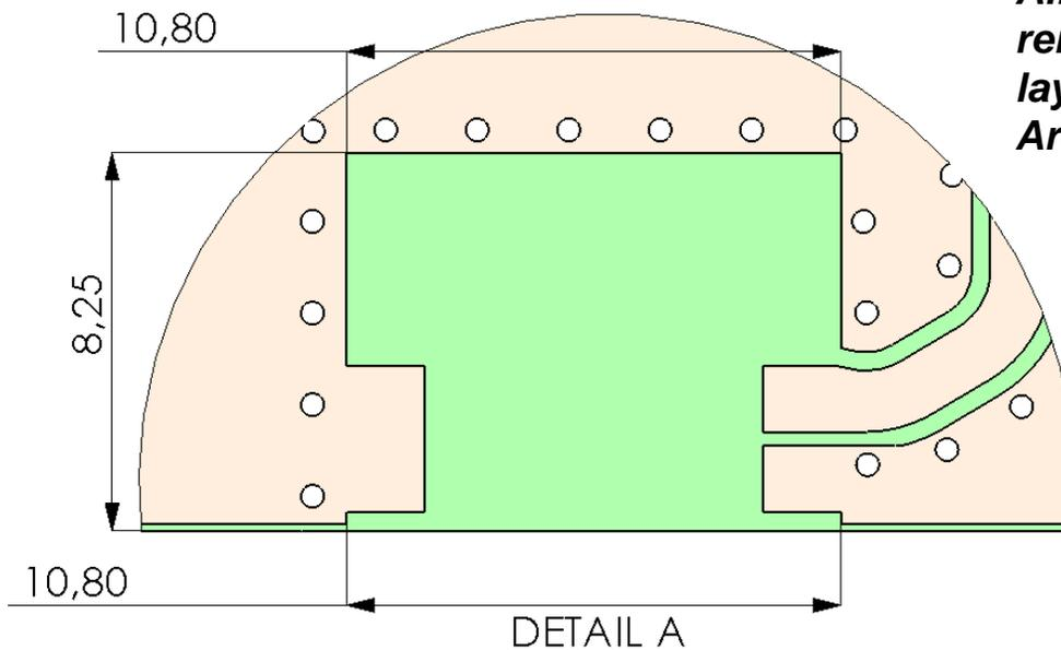
**All metallization must be removed from top and inner layers, clearance Area ( 10.8 x 8.25 mm )**
